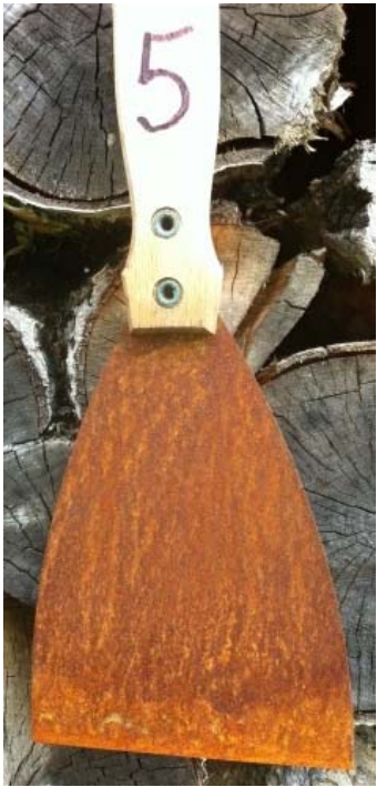
COYOTE SILKAL 93 SILICONE OIL HEAVY CORROSION
