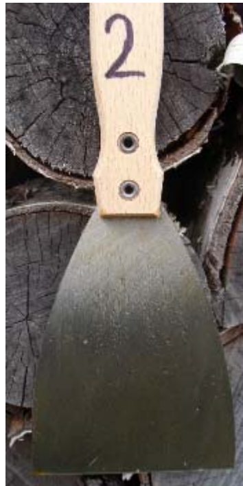
TECHNICAL VASELINE VERY VERY LITTLE CORROSION
