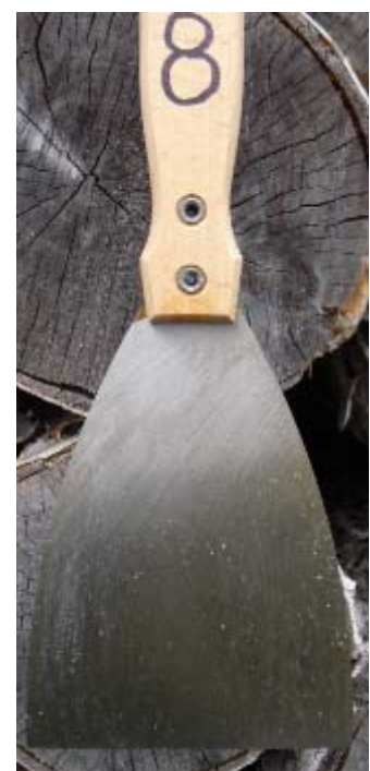
BERNER LUBRICANT AND ANTICORROSION VERY VERY LITTLE CORROSION
