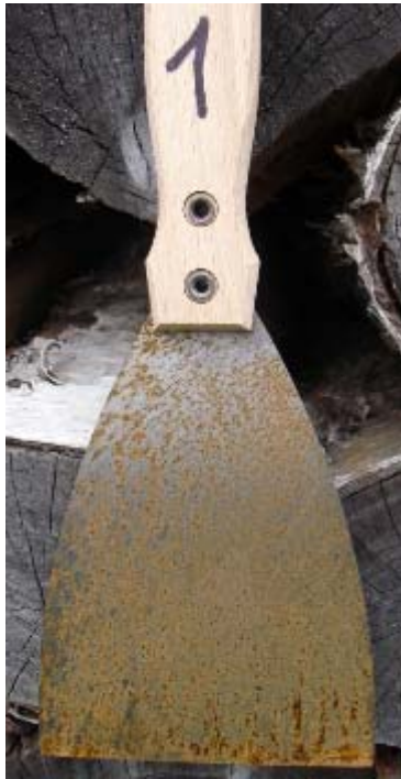
WITHOUT TREATMENT MEDIUM CORROSION
