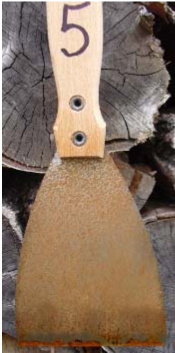
COYOTE SILKAL 93 SILICONE OIL HEAVY CORROSION
