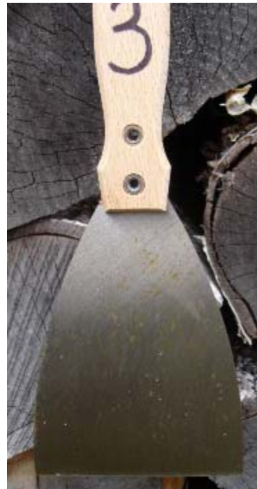
WD-40 MULTIFUNCTIONAL SPRAY LIGHT CORROSION
