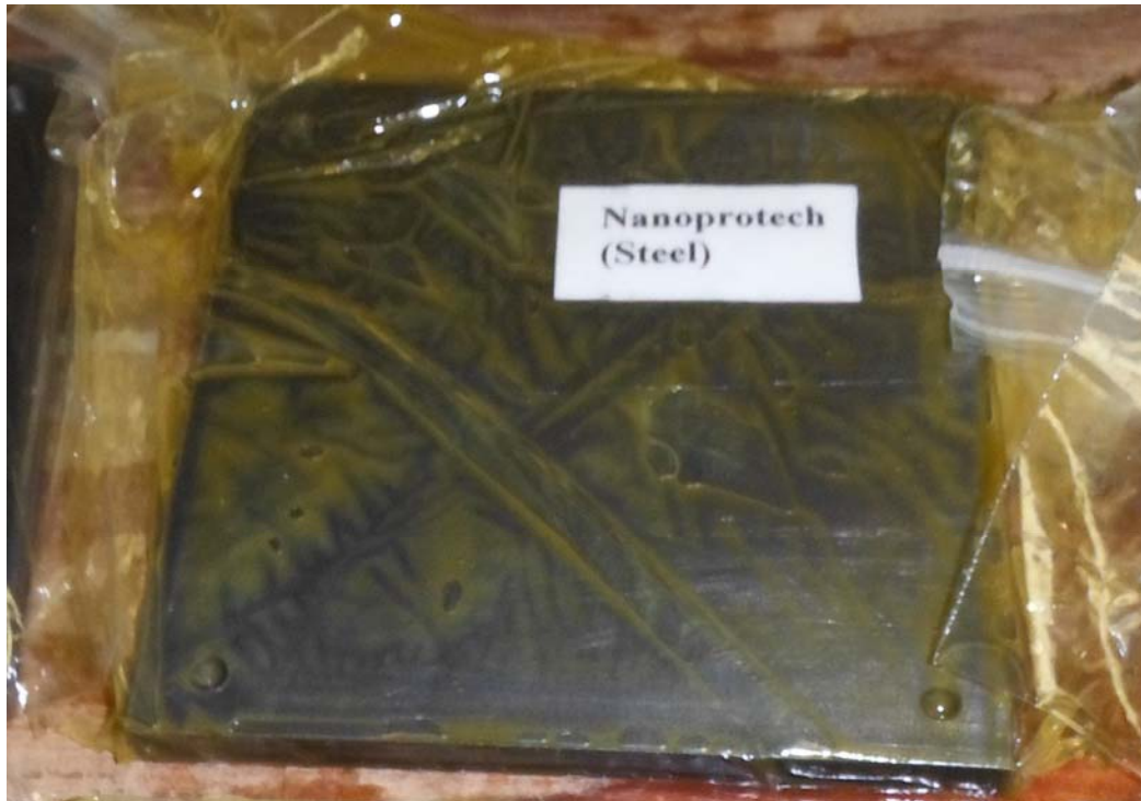
Figure 5: Nanoprotech Sample appearance prior to salt fog exposure
