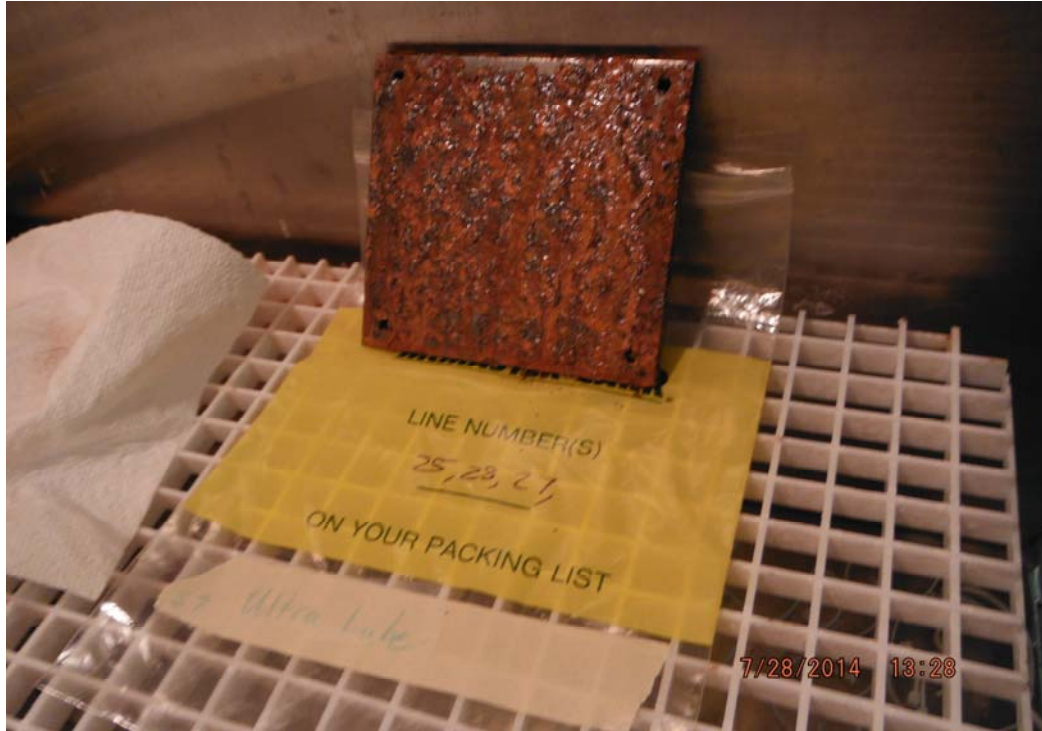
Figure 17: Steel Ultra Lube Sample appearance after completing salt fog exposure
