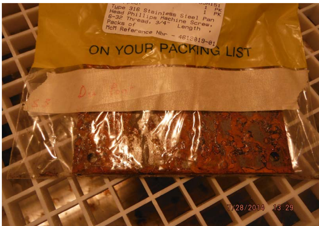
Figure 14: Steel DuPont Sample appearance after completing salt fog exposure
