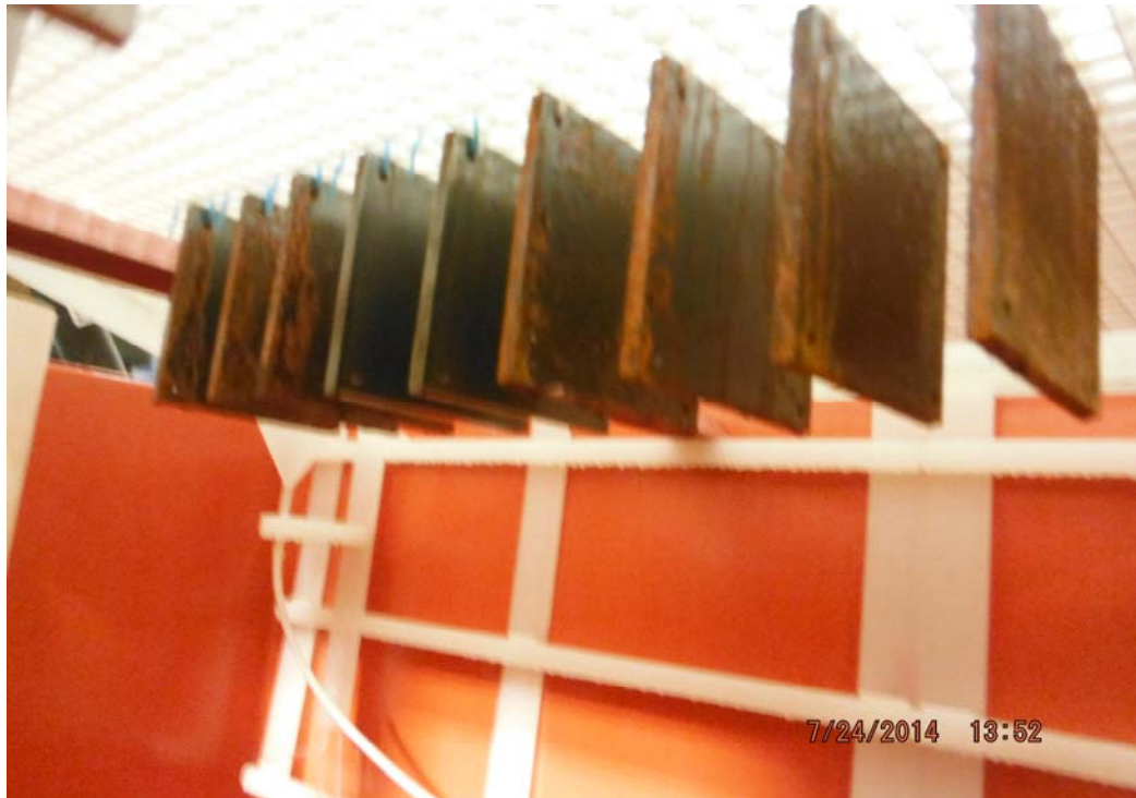
Figure 11: Test setup for the second forty-eight hours of salt fog exposure
