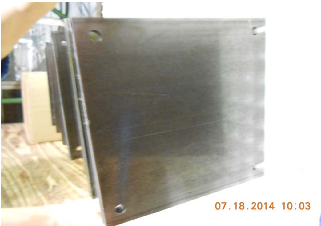
Figure 2: Liquid Wrench Sample appearance prior to salt fog exposure
