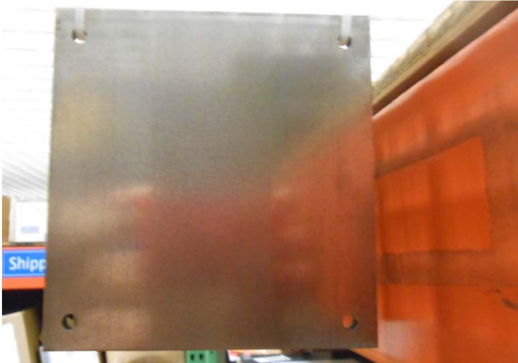
Figure 1: Control Sample appearance prior to salt fog exposure
