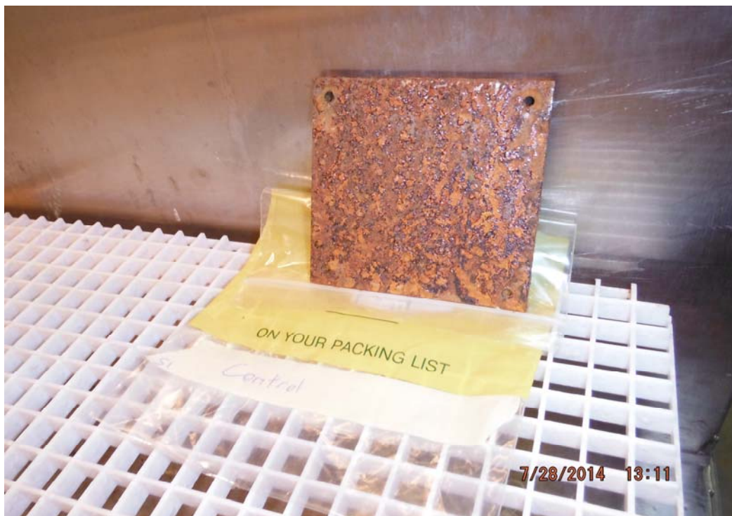
Figure 12: Steel Control Sample appearance after completing salt fog exposure
