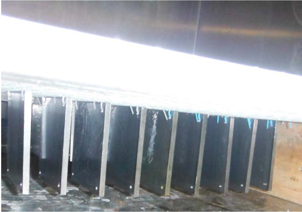
Figure 9: Test setup for the first forty-eight hours of salt fog exposure
