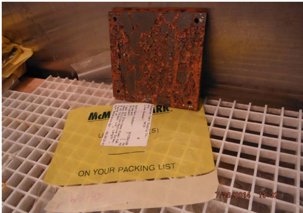
Figure 18: Steel WD-40 Sample appearance after completing salt fog exposure
