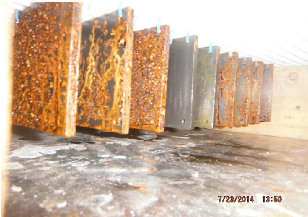
Figure 10: Coupon appearance after forty-eight hours of salt fog exposure
