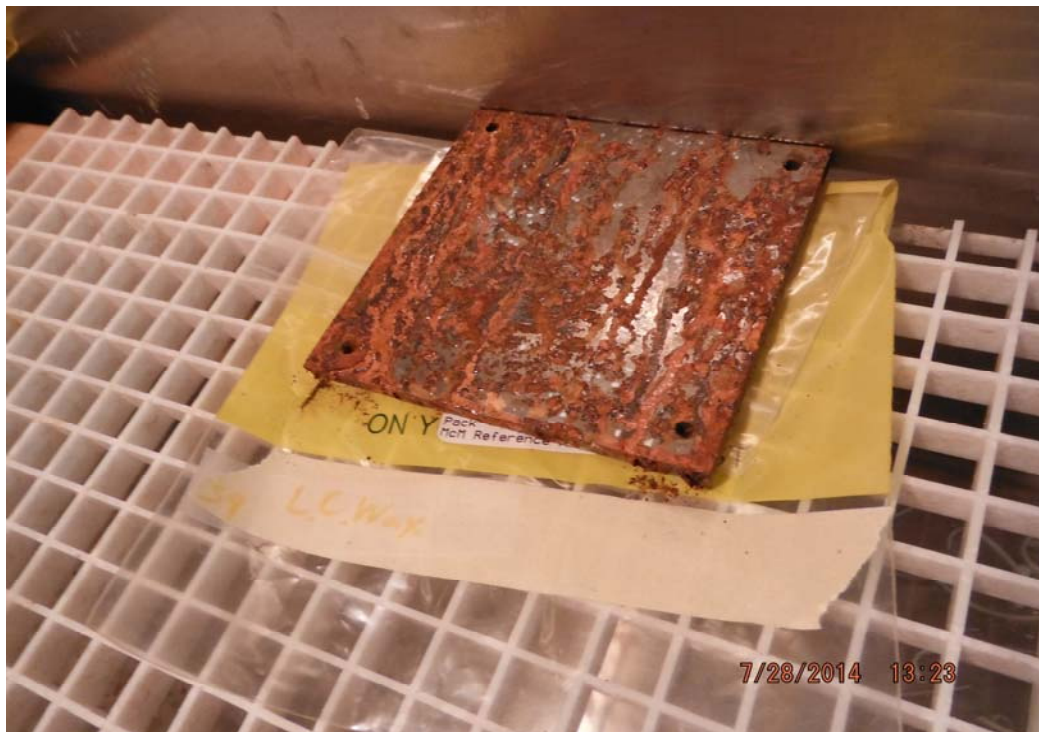
Figure 15: Steel L.C.Wax Alumaslick Sample appearance after completing salt fog exposure
